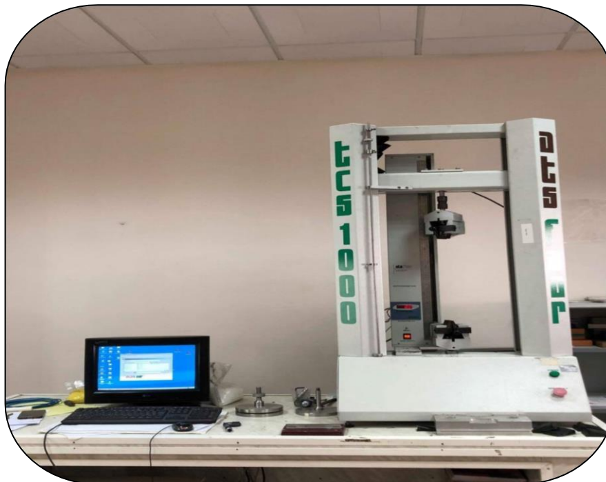
Figure II.2 Machine ATSFAR TCS 1000 de traction.
