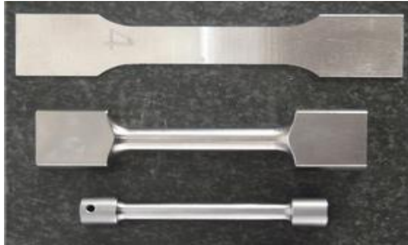
Figure II. 2: Eprouvette de traction uni axiale
